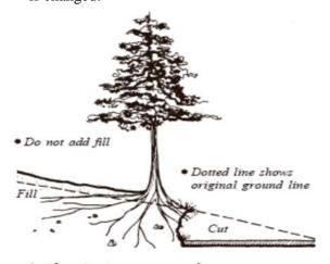
Avoid cutting into root zone close to trunk
